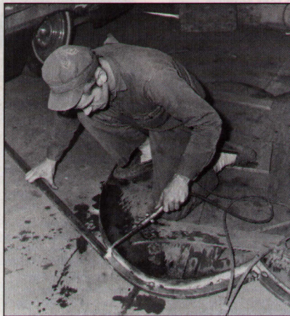
Returned from the bubble-blowing machine, the fresh bubble is ready to be marked and cut to the shape for Starliner's windshield. Note that the shape is defined with masking tape to prevent scratching, then cut with a fine-tooth bladed jigsaw.
